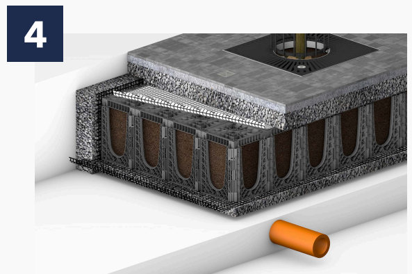
4 Cut and remove geocomposite.
