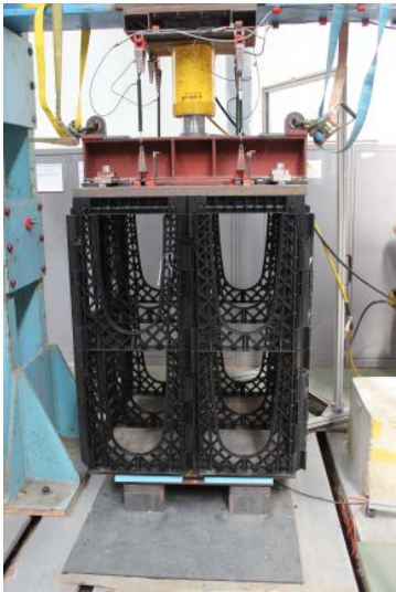
Photograph of RootSpace 600 (double height) being tested.
