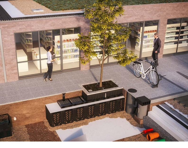
So how do we maximize uncompacted soil volume available for root growth without jeopardizing a stable base for sidewalks and roads? Soil support cells assemble underground to form a structural matrix filled with uncompacted soil to accommodate healthy root growth, while also providing a load-bearing structure for paved surfaces. They are the proven method for street trees, successfully implemented on thousands of projects around the world.
