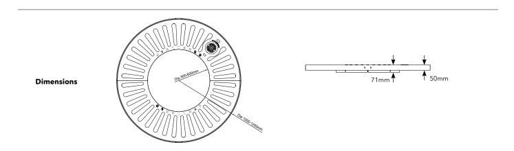
Vehicle Overrun Maximum 1.5 tonne SMWL (Slow Moving Wheel Load)
