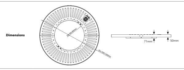
**Vehicle Overrun** Maximum 1.5 tonne SMWL (Slow Moving Wheel Load)
