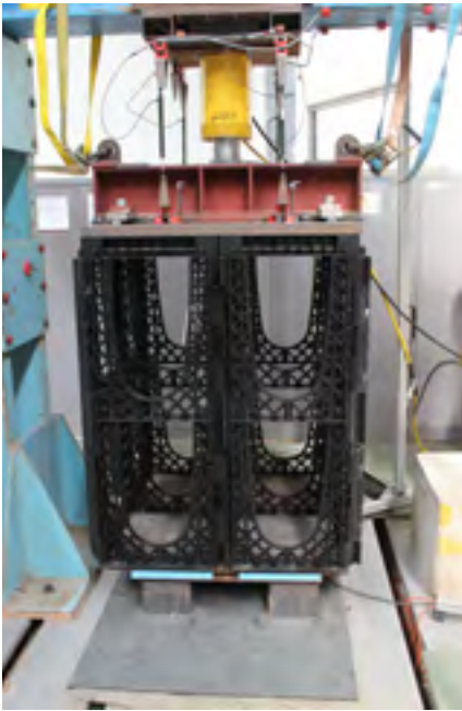
Photograph of RootSpace 600 (double height) being tested.
